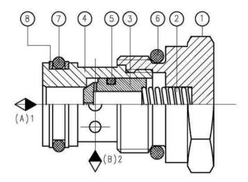
In throttling direction oil flows from connection A (B) to connection B (A) via a hole in poppet (3). Throttling depends on the hole diameter in the poppet (3). In the opposite direction oil flow acts on the surface face of the poppet (3).
