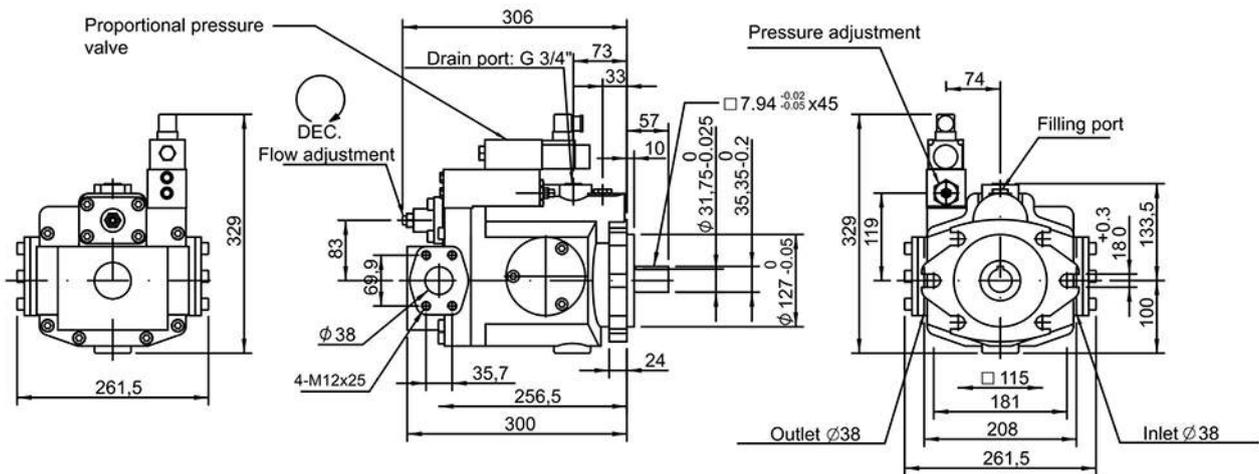
V50GR, V70GR Remote pressure compensator + Electrical unloading
