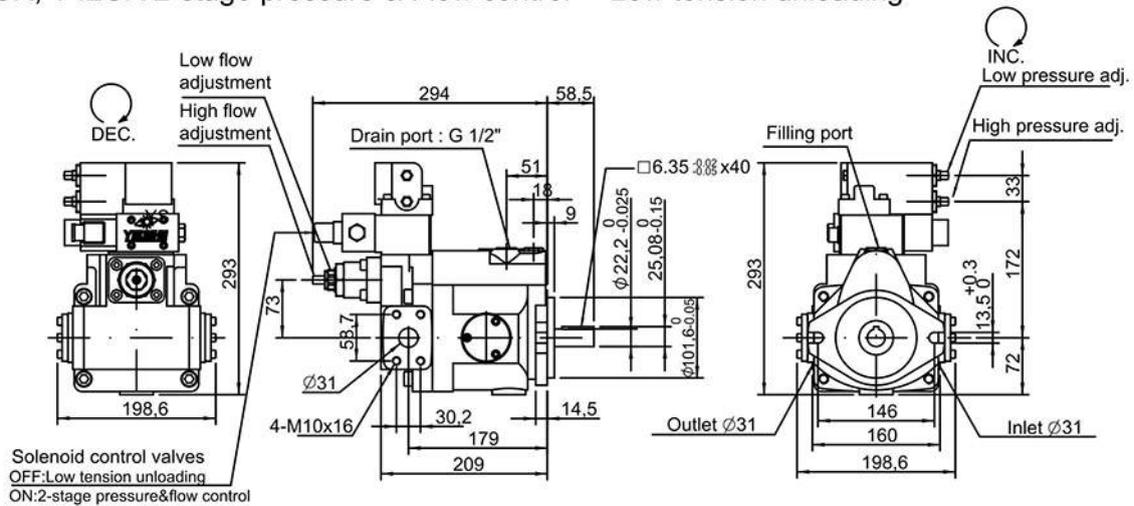
V38D, V42D Low tension unloading + Pressure control
