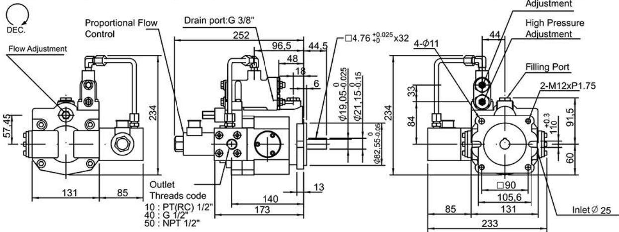
V15HK, V18HK Load-sensing compensator + Proportional pressure valve+ Proportional flow valve
