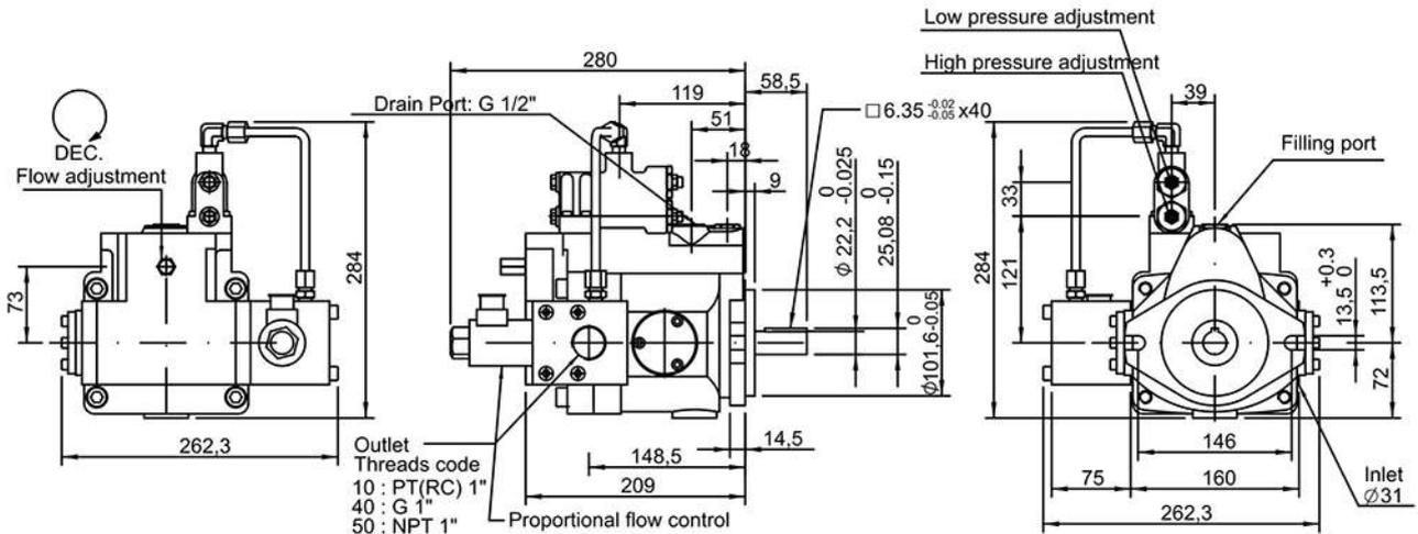
V38HK, V42HK Load-sensing compensator + Proportional pressure valve + Proportional flow valve
