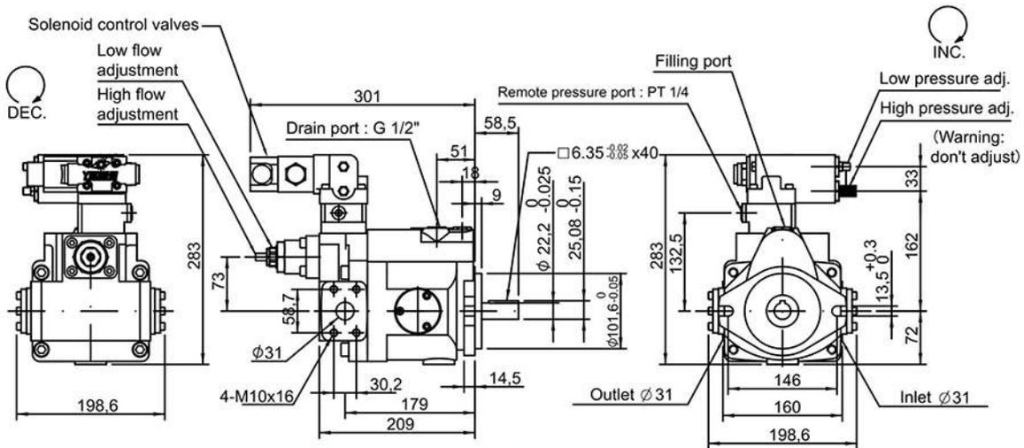
V38GM, V42GM Remote pressure compensator with NG6 interface
