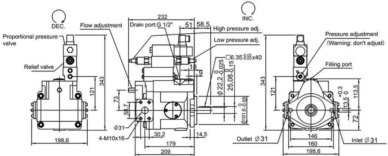
V38GC, V42GC Remote pressure compensator + Electrical unloading + 2-stage pressure control
