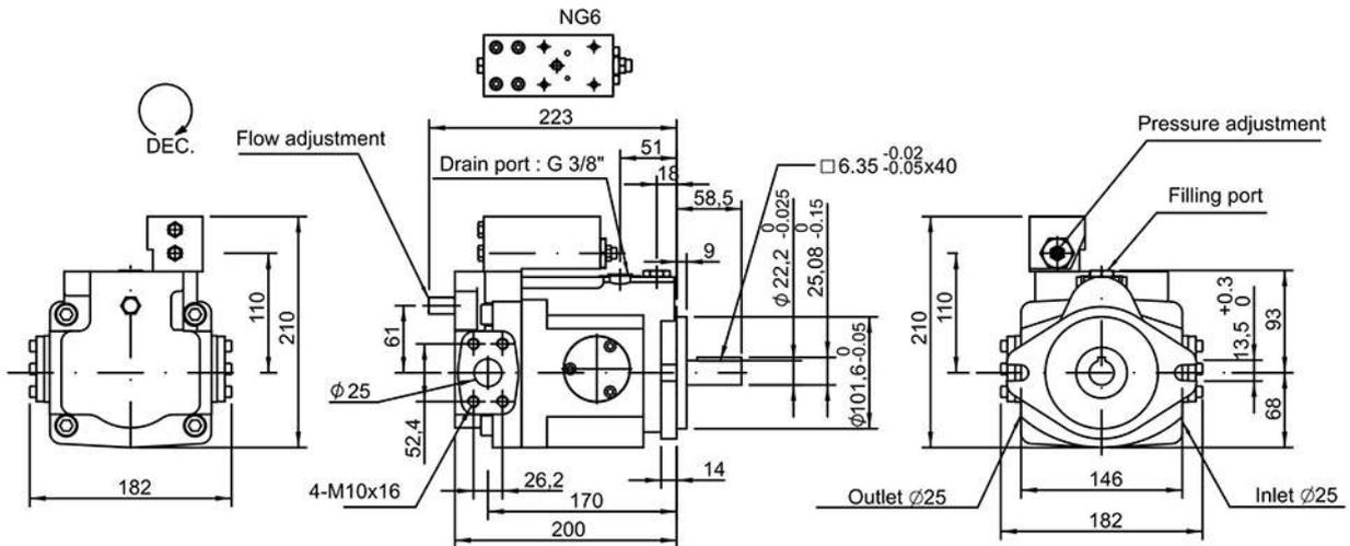
V23GJ, V25GJ Remote pressure compensator + Proportional pressure valve
