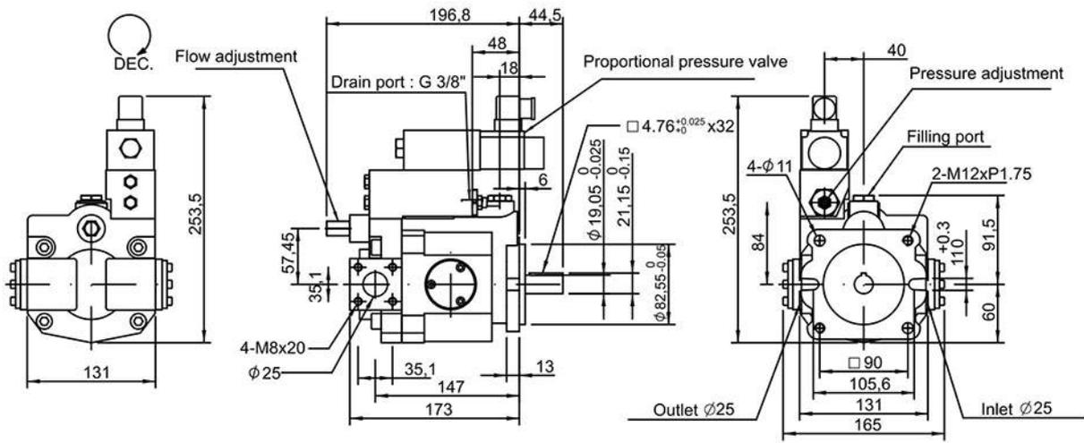
V15GR, V18GR Remote pressure compensator + Electrical unloading
