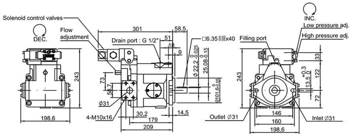
V38DG, V42DG Low tension unloading + Pressure control + Remote
