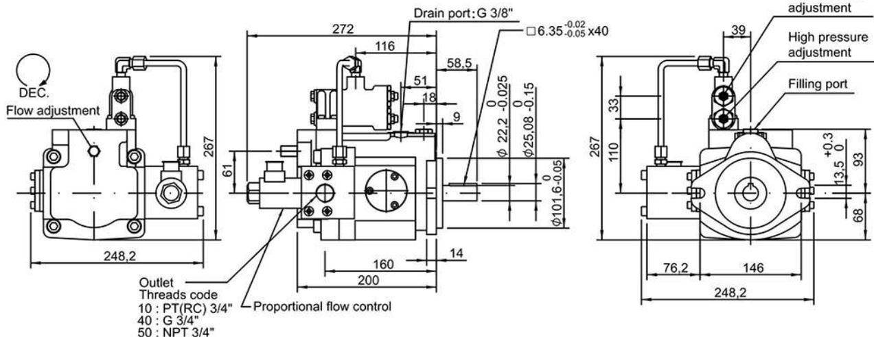
V23HK, V25HK Load-sensing compensator + Proportional pressure valve + Proportional flow valve
