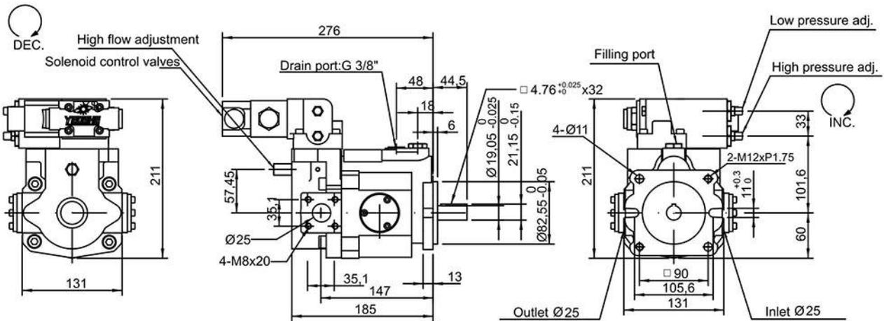
V15EG, V18EG Electric 2-stage pressure control + Remote
