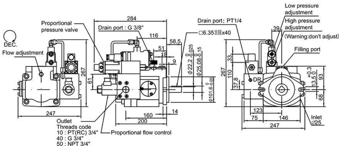
V23, V25 Thru drive(SAE A  $\phi 82.55$ , code D)
