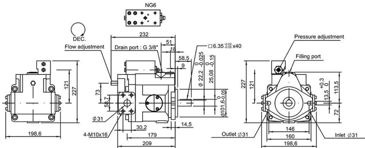
V38GJ, V42GJ Remote pressure compensator + Proportional pressure valve
