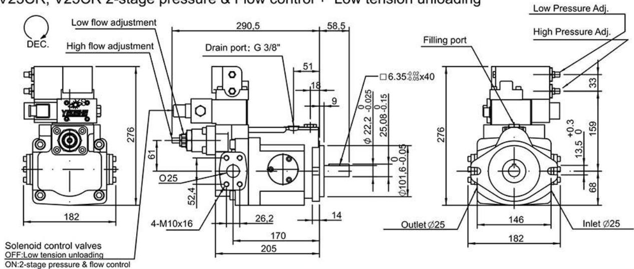
V23D, V25D Low tension unloading + Pressure control
