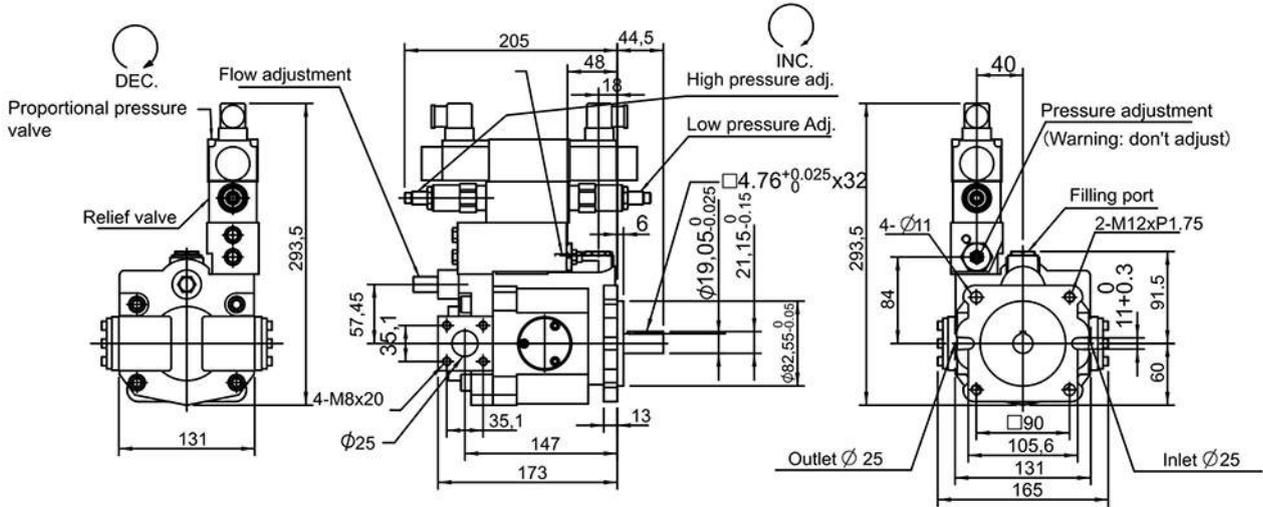
V15HQ, V18HQ Load-sensing compensator + Proportional flow valve+ Relief valve
