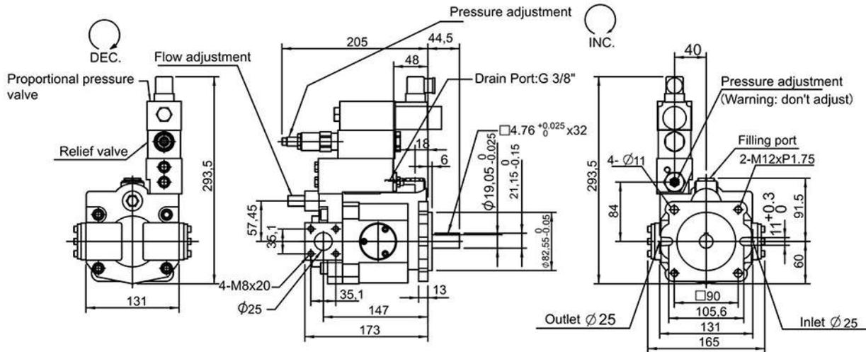
V15GB, V18GB Remote pressure compensator + 2-stage pressure control
