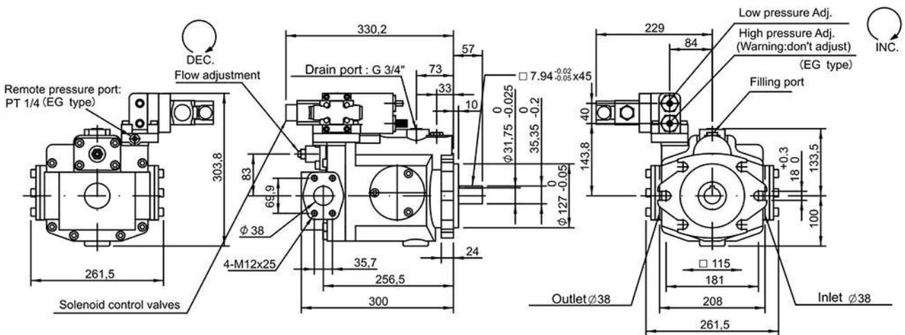
V50F, V70F Electric 2-stage pressure control & Flow control
